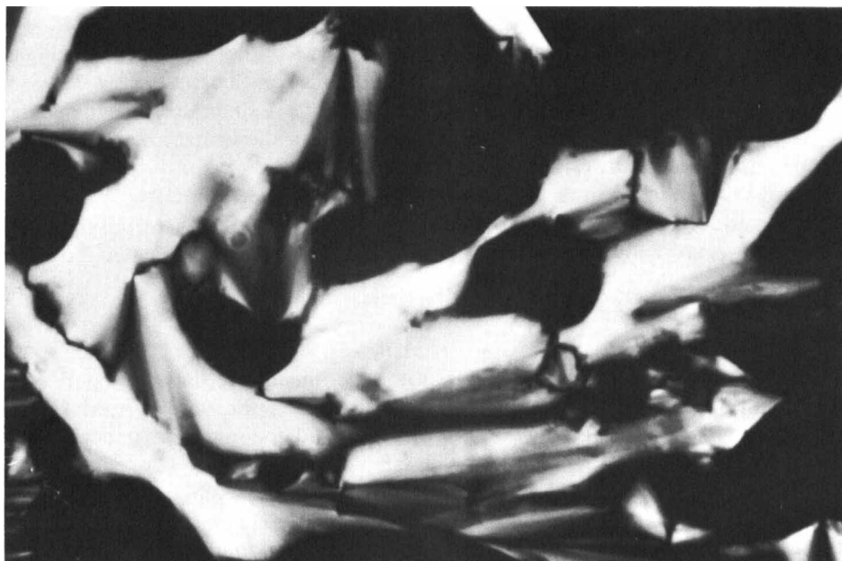
Figure 1. Focal conic and homeotropic textures of product (1) at 146°C (crossed polars, initial magnification 300×).
